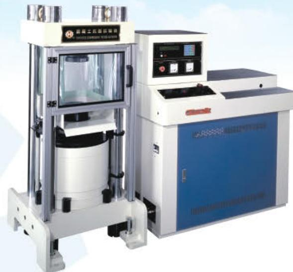
The machine adopts the HT-8336 Low Profile High Precision Load Cell sensor for measurement:
